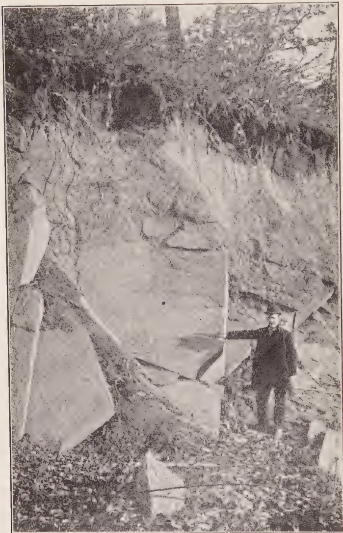
GNEISSIC GRANITE, GRADING FROM FIRM ROCK BELOW INTO WEATHERED ROCK AND SOIL ABOVE; ROCK CREEK PARK, WASHINGTON, DISTRICT OF COLUMBIA.
